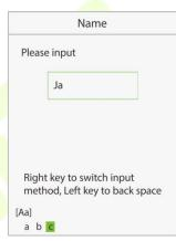
Press ► key to switch input methods: Mixed Case, Upper Case, Lower Case, Number, and Symbols.
