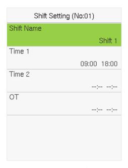
**Note:** The device supports a maximum of 24 shifts including two default shifts (Shift 1 and Shift 2). All the shifts are editable, and a single shift includes three-time ranges at most.
